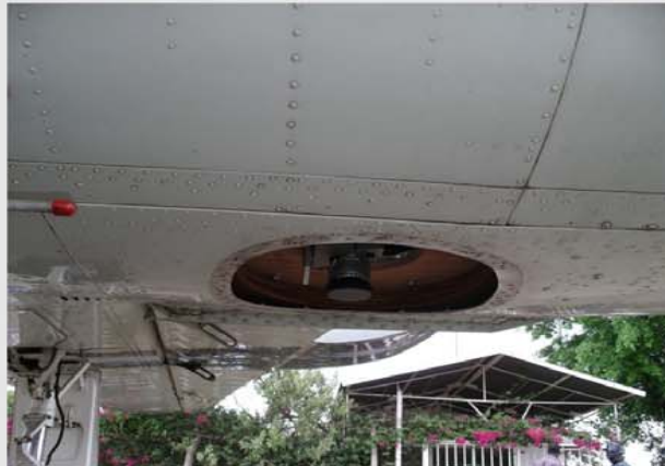
▲ Figure 4 FLIR ThermoCAM PM 695 mounted on aircraft PIPER NAVAJO, seen from outside the aircraft
